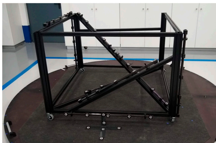
Figure 1. An arrangement of the reference scale bars for testing optical 3D measuring systems in accordance with VDI/VDE 2634 Part 1.
